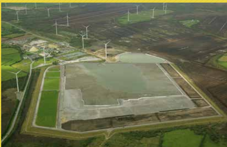
Rehabilitation and reclamation of closed tailing dam at Lisheen mine, Ireland.
