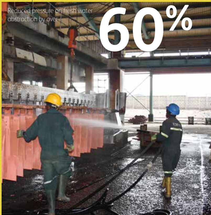
Recycled water getting used for washing copper plates at KCM, Zambia.
