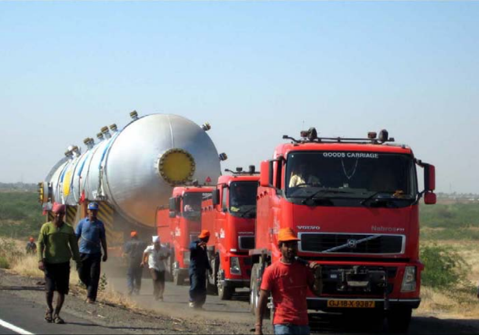
HDT Reactor Movement Ex-Kandla
